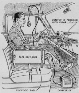
An office-in-the-car is easy to contrive with a tape recorder mounted on the front seat. To keep the recorder level, strap it to a plywood base having sides curved to the contour of the seat. It's a business-trip convenience to permit report dictation while held up in traffic.
