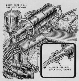
When rubber boots are used on ignitioncoil or distributor high-tension wires, you should push them all the way down on the tower. Otherwise the tendency of rubber to spring back into shape may force the wire out and break the connection.
