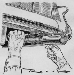
An exhaust deflector clamped on the end of the tailpipe is not just for looks. It is a good way to keep exhaust gases from discoloring your bumper chrome. Bushings are available for clamping a deflector to a small-diameter or oval tailpipe.
