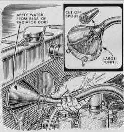
Cleaning radiator-core openings to free them of collected insects can be done without wetting the ignition. Cut off the spout of a funnel and adapt the top part to fit over the hose nozzle. Splashing water will be deflected back to the core and run harmlessly to the ground.
