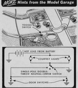
**Courtesy lights** or dome lights can be controlled with a three-way toggle switch in the circuit. On one side the switch gives you light while the doors are open; on the other the light remains on whether the doors are open or shut. The center position is at "off" at all times.
