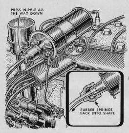
When rubber boots are used on ignitioncoil or distributor high-tension wires, you should push them all the way down on the tower. Otherwise the tendency of rubber to spring back into shape may force the wire out and break the connection.
