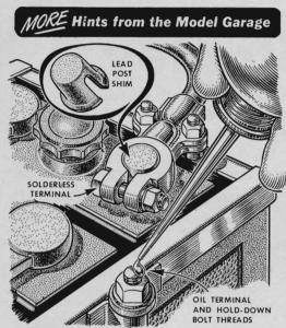
**Some battery tricks,** such as a spare solderless terminal to replace a broken one, may save you serious trouble on the road. An inexpensive lead shim permits tightening on a worn post. A drop of oil on the terminal and hold-down bolt threads every time you grease the car combats corrosion and makes battery removal easy.
