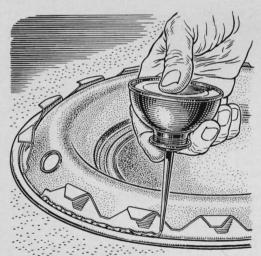
Wheel noises on cars having the new large-size hub caps are often caused by the caps themselves. Run a little brake fluid all around the inside crimp, prying gently with a screwdriver to let it all the way in, and you have a lasting cure.
