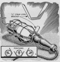
To keep a work light in place when you use it under the car, weld or bolt a bracket to the shield on the guard. It will then give light where you want it and won't roll from place. The flat sides allow concentration of light in any of three positions.
