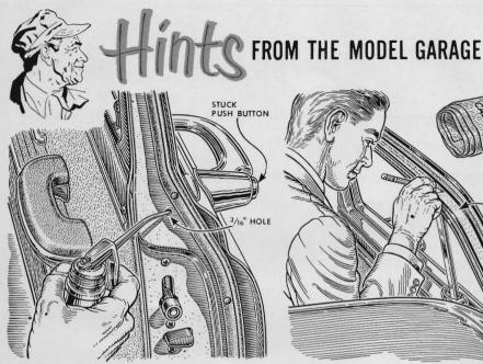
Freeing a stuck push button, on some cars requiring removal of the entire door panel, is easy if you drill the door edge in line with the latch contact. Squirt in penetrating oil to remove rust, then lubricate regularly with graphite.
