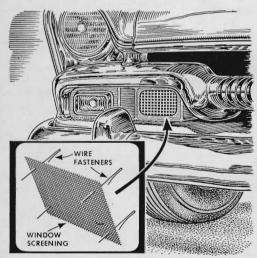
Window screening will keep small insects from getting into your car through the heater and ventilating air-inlet grilles. It can be fastened to the coarse-mesh openings with hooked wires pulled back through, as pictured in inset, and then twisted tight.
