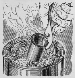
**Soaking a new radiator hose** in hot water helps to make it pliable. Then you can slip it more readily onto the radiator and cooling-system connections, especially when they are so close together that working with a stiff hose becomes a difficult job.
