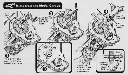
A Chevrolet timing gear can be replaced without removing the camshaft if you drill the hub opposite the keyway to weaken it so the web won't break under gear-puller pressure. Don't drill the shaft. Weaken further by driving in a tapered punch.
