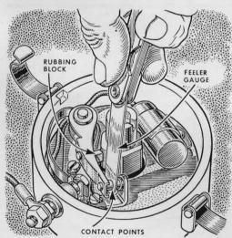
When you replace points, be sure to check the gap at intervals of around 1,000 miles until the fiber rubbing block shows a glaze. It wears rapidly until then, and may shorten the gap enough to make starting hard or burn the points.
