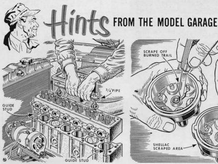
Tired of lifting overhead-valve heads for a succession of ring-and-valve jobs, one mechanic devised a convenient handle. Removing the rocker arms, he bolted a length of pipe to the brackets. Studs in hold-down bolt holes guided replacement.
