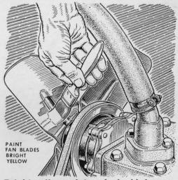
Bright-yellow paint on the fan blades may save you a cut hand. Painting the hood prop rod and its slot, too, will help you fit them together in the dark or dim light. The color has high visibility. Clean off all grease first so the paint will stick.
