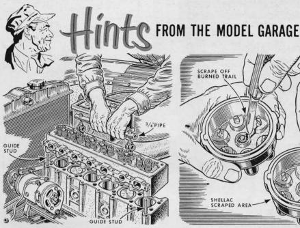
Tired of lifting overhead-valve heads for a succession of ring-and-valve jobs, one mechanic devised a convenient handle. Removing the rocker arms, he bolted a length of pipe to the brackets. Studs in hold-down bolt holes guided replacement.
