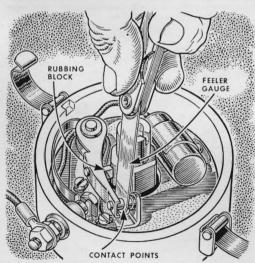
When you replace points, be sure to check the gap at intervals of around 1,000 miles until the fiber rubbing block shows a glaze. It wears rapidly until then, and may shorten the gap enough to make starting hard or burn the points.
