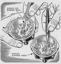
You can make a quick repair of a short in a distributor cap by scraping clean its telltale carbon trail between terminals and then coating the area with shellac. If all the carbon is removed, the shellac insulation should last a long time.
