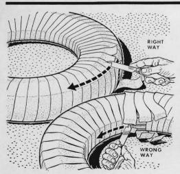
Wraps on tubeless tires should never be cut through between beads. It's bad practice on any tire, but with the tubeless type you stand the added chance of cutting the sealing area, causing a leak. Slice at the shoulder, where nicks are superficial.
