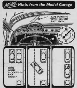
Parking in a tight spot is aided by an adhesive-tape marker on the dash shelf at a 7:07 o'clock angle. Stop parallel to the car ahead and about 18" away, turn wheel sharply clockwise, and back slowly until the marker points straight up the street. Cut all the way left, and back in.
