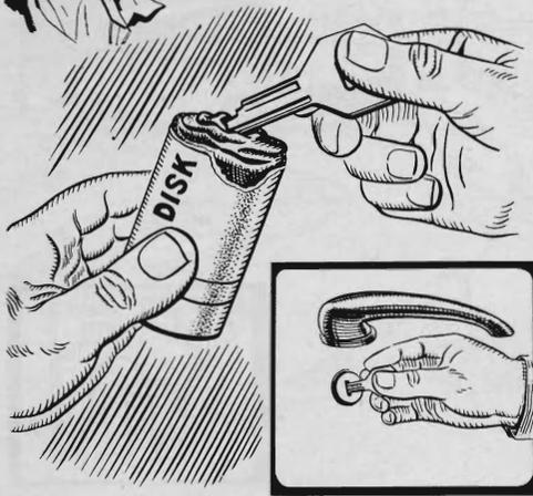
**When a key breaks off** in a car lock, try this trick. Smear the broken end with adhesive available from hardware stores for mounting sanding disks. Push the smeared end into the lock, then withdraw it. The adhesive may bring the tip out with it.
