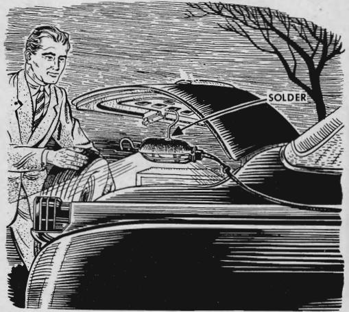
**A trouble light** usually has a hook only at the top, making it difficult to hang so that the light shines down. Solder a second hook to the back of the reflector, as above, and you will find that the light will be much more convenient to use.
