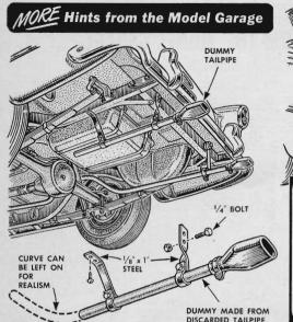
That dual-exhaust effect for the going-away view can be produced this way if you don't want the real thing. Scrounge around an auto junk yard until you find a suitable tailpipe. Then bracket it opposite the real one and clamp on twin chrome extensions.
