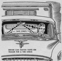
When a trailer has a flat, it's hard to see it from the tow car. Place two strips of tape on the trailer front where you can see them in the rear-view mirror just above the lower edge of the car window. If a strip drops out of sight you know there's a flat.
