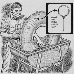
To mark leaks in tubes, one garageman twists skewer-shaped pins from stiff wire. He hangs them on a peg near the test tub and inserts one in each puncture he finds. When he gets around to repairing the tube, he replaces the pins on the peg.
