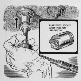
**Hard undercoating** makes it difficult to remove body and fender bolts from a car that has had a heavy application. To speed the operation, one shop owner uses sockets ground to a sharp edge like this. The knife edge cuts right through the coating.
