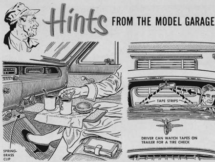
A handy snack table for two is easy to make from an old sun visor. Position and bolt the bracket to the dash so that the visor swings under it when not in use. Use a second, U-shaped bracket to support the downward-hinging edge of the extended visor.
