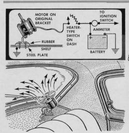
For a rear-window defroster, attach an old car-heater fan to the parcel shelf. Cushion it with rubber. Use a grounded metal plate under the shelf as a screw anchor. Rig a variable-resistance switch on the hot side of the ammeter to feed the motor.
