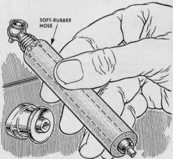
A tire gauge carried in a toolbox or the glove compartment will be protected and won't cause an annoying rattle if you locate rubber hose of the right diameter, cut off a piece and slip it on the gauge. You can take readings without removing it.
