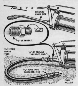
A grease gun will reach all fittings with ease if you replace the rigid-nozzle tube with a '49 Ford flexible brake line. Attach the line to the gun with a tube fitting having a ''' pipe thread on one end and a '''-24 thread on the other. Screw the original grease-gun nozzle on the male ''' pipe thread on the free end of the brake line.
