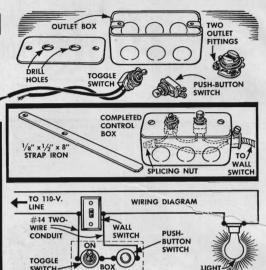
wire armored cable links the automatic control box to the wall switch box in an outand-back circuit. Connections in the wall switch box are made at the switch-terminal screws. Remove a knockout plug to admit the wires and clamp them to the box.
