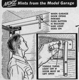
The light goes on automatically when you open a garage door equipped with this setup—just as in a refrigerator. Close the door and it goes out. A normally closed, spring pushbutton switch operated by a strap-iron finger on the door does the trick. A length of two-
