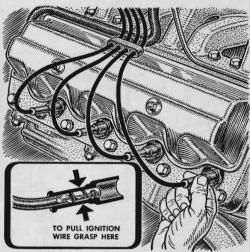
When cleaning or changing spark plugs, owners of Plymouth V-8s should pull the ignition wires by grasping them only at the reinforced section near the plug. Pulling on the wire might cause an internal break resulting in misfiring or weak spark.
