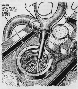
Check your battery water more often than usual during the hot late-summer days. The water evaporates faster in the excessive heat and can drop below the top of the plates in a week's time, drying them out and reducing output. Maintain the water level %" to %" above the plates, but don't overfill as it will bubble out of the vents.
