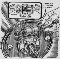
Clean wheel cylinders thoroughly when installing new brake linings. The full thickness of the new lining will push the cups deeper into the cylinder, and gum or dirt on this long-unused part of the wall may cause the cylinder to leak. Be sure to use only hydraulic-brake cleaning fluid, and allow to dry before reassembling parts.
