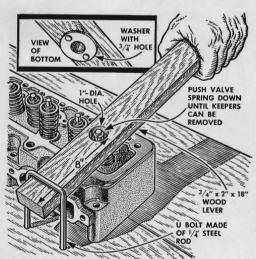
Valve springs on overhead-valve engines can be compressed and held safely while the keepers are removed by using a piece of hardwood as a lever. Place the head on a heavy board and fasten a U bolt in position behind it. Shift the head after each spring is removed to align the next valve with the U bolt. Reverse procedure to install valves.
