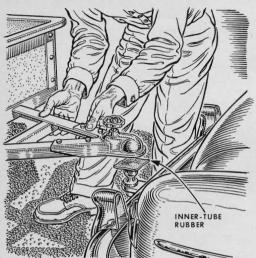
Rubber padding in the socket joint of the hitch will give you a nonrattling coupling that won't click and jerk when you pull a light trailer. Just lay a square of old inner-tube rubber on the ball before dropping the hitch on it.
