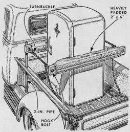
Heavy, padded braces at front and back prevent slipping and scuffing when you move a partial load in a truck. Link the holding chains as taut as possible to the free-riding rear brace, then tighten with the turnbuckles to hold the load fast.
