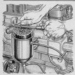
Two screwdrivers, with the handle of one used as a fulcrum, provide the leverage you need to start a stuck oil-filter refill without yanking off the wire handle. Take care not to nick the sealing seat of the housing, or leakage may result.
