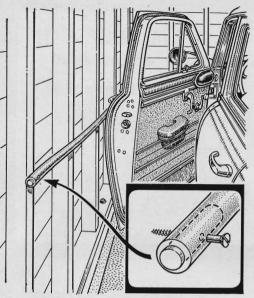
Discarded garden hose used as a bumper on your garage wall protects the car door when you open it to get in or out. Drive a short dowel in each end and drill for a mounting nail or screw. Use a concrete nail or expansion bolt in a masonry wall,
