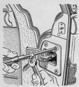
**Turning a screwdriver** while tightening or removing a door hinge can be made easier if you braze a nut on the shank near the handle. Then put pressure on the end of the screwdriver and do the turning with a small open-end wrench.
