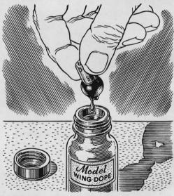
**Model-airplane dope** or fingernail polish will cut down annoying glare from dash lights. Simply dip the bulbs in the red dope and let dry. Then, checking as you work, start at bottom and gradually scrape off coating until light level is just right.
