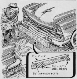
Bumper and grille protection when you are called upon to push-or need pushingis carried in your trunk with a guard made from a short length of stout lumber. Bend and bolt on the steel straps so that they fit loosely over the bumper guards.
