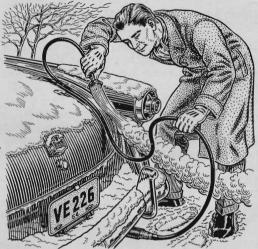
An ordinary shower hose, with spray head attached, makes quick work of thawing out a frozen trunk lid to get at the chains and jack. With the faucet attachment slipped into the exhaust pipe, hot engine gases melt the ice without damaging paint.
