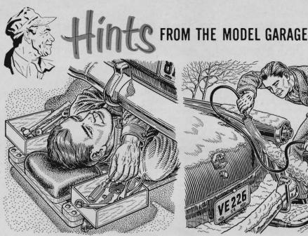
Attach a cigar box to each side of a creeper headrest to hold wrenches, screwdrivers and other small repair equipment. Kept in the boxes, the tools will always be within easy reach, no matter how much you move around on the creeper.
