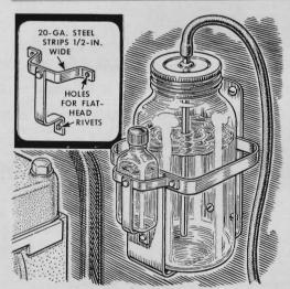
Make a small metal cradle and attach it to the side of your windshield-wiper reservoir bracket to hold that little bottle of solvent antifreeze that's always getting lost or broken. The cradle is held together and to the bracket with flathead rivets.
