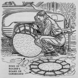
Store tire chains on disks of heavy cardboard or wallboard cut to the outside diameter of the tires. Free from kinks and easy to handle, the chains can be brought up alongside the wheels and transferred from the disks to the tires in short order.
