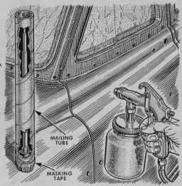
A mailing tube can save you the trouble of masking your car's radio antenna next time you want to do a partial or complete body refinishing job. Just slip the tube over the end of the telescoped antenna.
