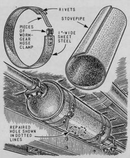
Patch a leaky muffler with a length of stovepipe clamped around it this way. Cut apart two aircraft-type hose clamps and rivet the pieces to two metal bands as shown. Slip the bands around the stovepipe and pull up tight with a screwdriver.
