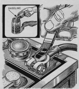
**Stop battery corrosion** around posts and terminals with a paint made from the pitch of old batteries dissolved in gasoline. The paint can be stored in a closed jar and brushed on whenever the cables have been removed or a new battery is installed.
