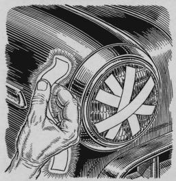
A roll of reflective tape, carried in the glove compartment, will protect you against collision if you're caught with a dead headlight. Strips pasted across the lens will show other motorists which light is out so that they can pass at a safe distance.
