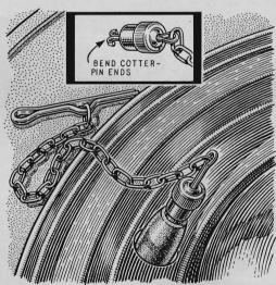
One way of holding a valve stem when mounting a tire is suggested here. Screw on the chained valve cap after inserting the stem through the rim hole. If the stem slips back, the cotter pin on the end of the furnace chain won't let it go too far.
