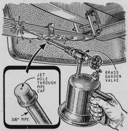
Oiling hard-to-reach spots is easy with this pressure lubricator made from an ordinary blowtorch. Unscrew the burner and screw in the nozzle made from a valve and two lengths of pipe as shown. Pumped up, the rig will squirt oil several feet.
