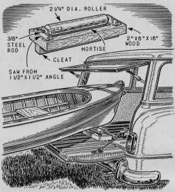
Loading a boat into a station wagon is an easy one-man job with this roller that slips quickly between tailgate and body. The roller can be from an old lawn mower or kitchen rolling pin, mounted as shown.
