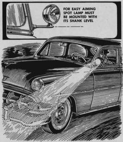
When mounting a spotlight, be sure to get the control arm level so the beam will stay level as you swing it. Wire the spotlight independently of the head lamps so that if the latter should fail, you still will be able to continue.
