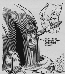
Tail lights will shine brighter if you paint the inside of the lamp receptacles with white enamel to increase their reflectivity. This is especially helpful on older cars where the housings have become heavily rusted. Clean the metal thoroughly before painting.
