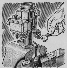
To hold a carburetor while you work on it, clamp two %" bolts in a vise and bolt the carburetor to these through the mounting holes in the flange. This will provide a very rigid work mount without danger of damaging the carburetor.
