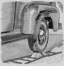
Tire chains can be quickly put on without jacking up the car with this ramp made from a 4"-by-4" notched in the middle. One cross link is laid in the notch and the wheel driven on top, leaving the chains loose at the bottom and easy to clasp.
