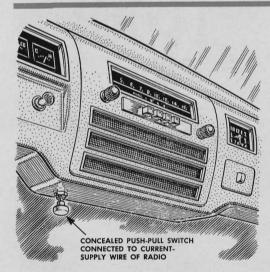
A car radio can be turned on and off without disturbing the volume control if you wire a separate push-pull switch in ahead of the regular one on the control. Position of the knob under the dashboard also helps prevent unauthorized use.
