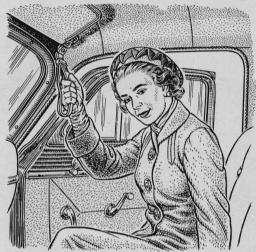
An extra hand strap added to the right front seat will make it easier to get in and out, and provide a handhold on rough and curving roads. Securing the strap to one of the screws that hold the sunshade bracket saves drilling new holes.
