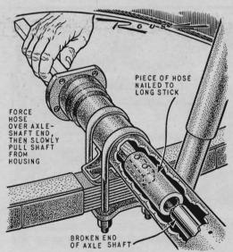
Tack a short piece of radiator hose to a stick to fish out the remaining stub of a broken axle shaft. Try different sizes of hose on the broken end of the piece that came out of the housing to find a diameter that will fit snug enough to do the job.
