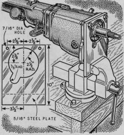
**Support a '49-'54 Ford transmission** for easy overhaul by bolting it to a heavy steel plate clamped in a bench vise. The large opening gives access to the bolts holding the main-shaft bearing retainer and the small opening permits removal of the countershaft.
