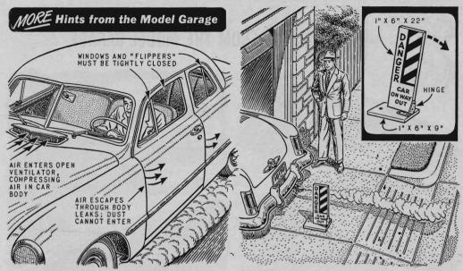
In dusty driving, it helps to close all windows and open the cowl or heater vents wide. This raises the air pressure inside the car. If the windows are partly open, pressure is reduced and dust is sucked through the seams and body openings.
