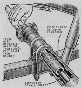
Tack a short piece of radiator hose to a stick to fish out the remaining stub of a broken axle shaft. Try different sizes of hose on the broken end of the piece that came out of the housing to find a diameter that will fit snug enough to do the job.
