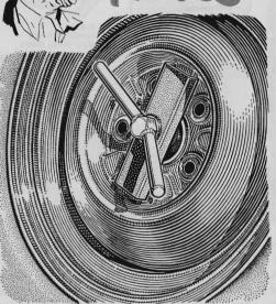
A spare-wheel nut becomes a quick-acting wrench for removing and mounting the spare in the luggage compartment when two 3½" lengths of ½" rod are welded to it to form a handle. The handles also reduce the chances of the nut rolling out of sight.
