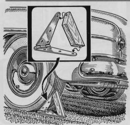
A collapsible wheel chock may save your car from an unexpected take-off when changing a tire. A nail protruding from each end of the wooden brace fits into the end screw holes of the strap hinge to hold it open. The chock folds flat for storage.
