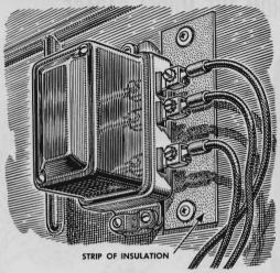
A possible cause of shorts is small clearance between the voltage-regulator terminals and the metal fire wall of a car. A strip of gasket material fastened to the fire wall behind the terminals will prevent shorts from bent terminals or oversize bolts. A tire patch cemented to the fire wall could also be used.
