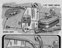
A stainless-steel plate fitted between the armrest and the door upholstery will save the fabric from wearing or cover an already worn spot. Slip the upper edge of the plate under the decorative molding strip and hold it in place with the armrest screws.
