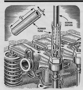
A length of rubber tubing slipped over your screwdriver will hold the tool in the slot while you adjust bouncing valve tappets. The hose fits over the adjusting screw and leaves the lock nut exposed for tightening when the right setting is made.
