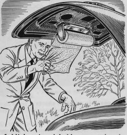
A kitchen towel holder mounted under the deck lid with self-tapping screws will speed clean-up operation after you make roadside repairs or change tires. Keep waterless hand cleaner in the trunk to loosen the grime before wiping.
