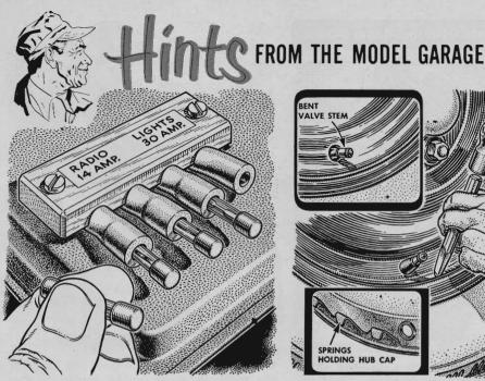
Tuck spare fuses into a clip made from short lengths of windshield-wiper hose for quick replacement as needed. A notched wood block screwed to the inside of the glove-compartment door holds the hose.
