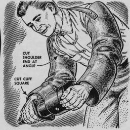
Join two pieces of inner tube with a leather strap to make a pair of sleeves that will protect your arms from dirt or a hot manifold when reaching in or around the lower parts of a motor. Use the sleeves for protection against sparks when welding.
