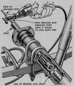
Use welding rods to remove broken axle stubs. Tack two rods end-to-end. Clip one electric welder clamp to a rear spring, the other to the rod. Make a pass at the stub through a piece of garden hose. Welded to the rod, the stub is pulled out easily.
