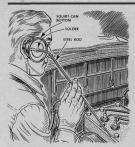
Locate hard-to-find engine knocks with a homemade stethoscope. Make a right-angle bend near one end of a curtain rod, and solder this end to the bottom of an oil can. Probe the engine block with the rod, holding the can mouth to your ear. Diaphragm-amplified sound is easily spotted.
