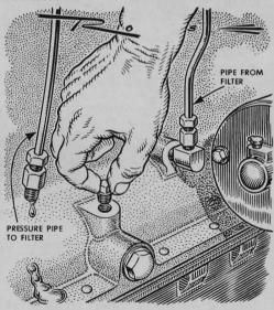
The right-size pipe plug, stored in your car's tool chest, can save you a lot of trouble if a bypass-type oil filter or its lines develop a leak out on the road. Remove the inlet tube where it couples to the engine block, insert the plug, and your emergency repair will get you home.
