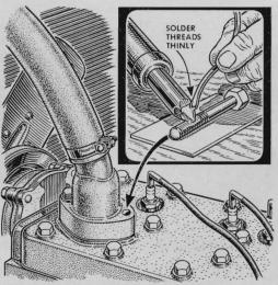
Stop leaks around bolt threads that can't be sealed with new gaskets by removing the bolts and floating soft solder over the threaded area with a soldering iron or torch. Leave the first few threads untinned for easy bolt replacement.
