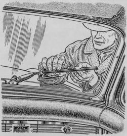
Caught in bad weather with a wiper blade that doesn't clean the windshield well, try switching it with the one on the passenger's side. Chances are the right-hand blade is in better shape; it gets less mud and sand tossed at it by passing cars.
