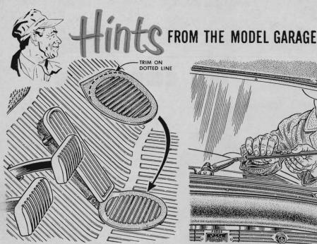
Shoe-sole repair kit, which can be bought in most five-and-dime stores, gives you the makings of a first-rate patch for that wornout section of floor covering under the gas pedal. Trim one of the rubber soles, as shown, and cement it firmly in place.
