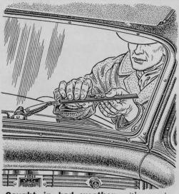
Caught in bad weather with a wiper blade that doesn't clean the windshield well, try switching it with the one on the passenger's side. Chances are the right-hand blade is in better shape; it gets less mud and sand tossed at it by passing cars.
