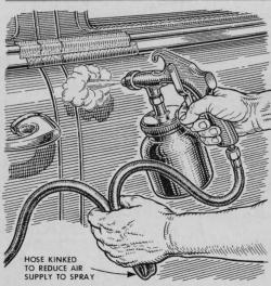
Save time on touch-up paint-spray jobs by kinking the air hose slightly with the left hand to reduce paint-spray volume temporarily. It's easier than making numerous adjustments on the air regulator to prevent overspray and time-taking clean-up jobs.
