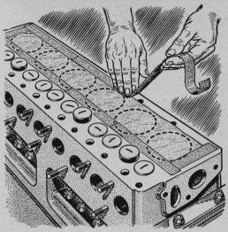
Cover cylinder bores before you grind L head engine valves. Otherwise, damaging grit may get in. Use wrapping paper to cover the bores, attaching it to the block with masking tape. After valves are ground, brush away grit before removing the paper.
