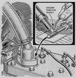
Stop leaks around bolt threads that can't be sealed with new gaskets by removing the bolts and floating soft solder over the threaded area with a soldering iron or torch. Leave the first few threads untinned for easy bolt replacement.
