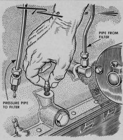
The right-size pipe plug, stored in your car's tool chest, can save you a lot of trouble if a bypass-type oil filter or its lines develop a leak out on the road. Remove the inlet tube where it couples to the engine block, insert the plug, and your emergency repair will get you home.
