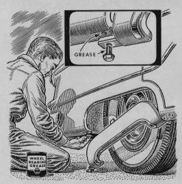
Make fender skirts easy to remove by coating the lock bolts with heavy wheelbearing grease to keep them from rusting. Skirts are bolted on many late-model cars and it is almost impossible to remove a rusted-tight nut without twisting or otherwise damaging the fender.
