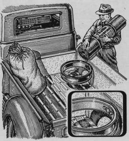
Bolt one or two truck-tire rims to the side of a pickup truck to keep cylindrical objects like oil drums or rolls of roofing from rolling about. Bolt the rims as high up from the floor as the sides will permit to keep the loads from tipping out.
