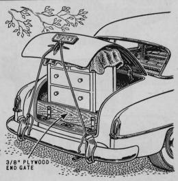
Put a plywood end gate across a low trunk opening to keep tools from rolling out when transporting a large object with the trunk lid up. Set it back far enough so that it won't interfere with the latch and secure it with metal angles bolted to the floor.
