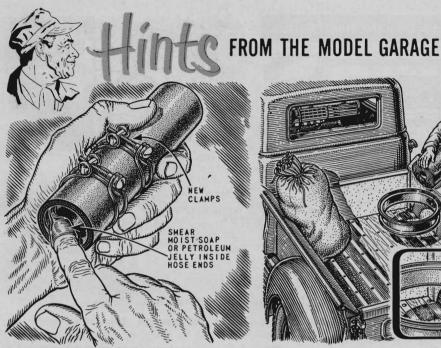
Rub soap inside hose ends when installing new connections between the radiator and motor block. They'll slip on the fittings easily and save you much pulling and tugging. For a thorough job, sandpaper the rust off the fittings and use new clamps.
