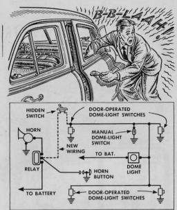
A simple and effective burglar alarm can be installed with a length of wire and a single-pole switch. Use the wire to connect the horn and courtesy-light circuits through the switch. If anyone opens the door, the horn will blow. Hide the switch somewhere on the exterior of the car so you can shut off the alarm system.
