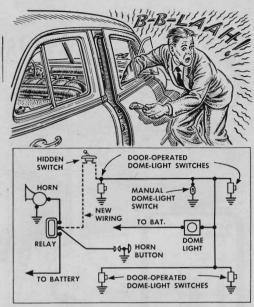
A simple and effective burglar alarm can be installed with a length of wire and a single-pole switch. Use the wire to connect the horn and courtesy-light circuits through the switch. If anyone opens the door, the horn will blow. Hide the switch somewhere on the exterior of the car so you can shut off the alarm system.
