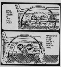
How high you sit may determine whether you have a clear view of the driving gauges through the steering wheel. On late cars with two-spoke wheels it sometimes helps to pull off the wheel, turn it 180° and remount it with the spokes below the center.
