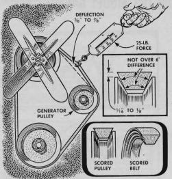
Fan-belt life may be shortened by any of the reasons indicated here. In installing a new belt, always make sure it is engineered (in cross section) to fit your particular pulleys. If a pulley is scored, your belt eventually will become scored too—and weakened. If too tight, the belt will damage water-pump and fan bearings.
