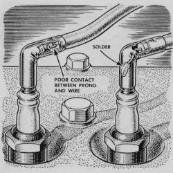
Hard starting may result from a faulty contact between the spark-plug wire and connector. In such cases, one mechanic suggests stripping back the insulation, replacing the connector and soldering the bare wire to the side of the connector.
