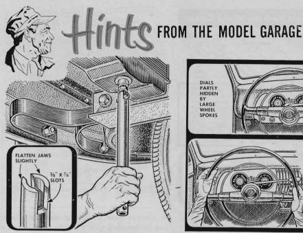
A wrench made from hardened copper tubing makes it easier to open and close a cooling-system petcock under the car. As you open the petcock, the coolant will run down the tubing, not your sleeve. Drill a hole in the end and hang it on a nail.
