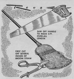
A handy brush for cleaning road dirt from the underside of a car can be made from a discarded household broom. Shorten the handle with a saw and snip about 6" off the bristles, leaving just enough so you'll have a brush that's good and stiff.
