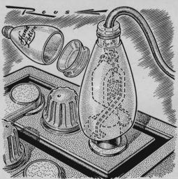
In working with several batteries around a shop, there's always a chance the clamps may contact other conductors. Insulating shields for the clamps are easily made from the flexible plastic bottles used for cosmetic sprays and the like.
