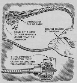
**Speedometer noise** may result if relative lengths of the cable and casing are not correct. The sketch shows how much the cable usually should extend from the casing at each end. Twisting the casing will shorten or lengthen it as much as ¼".
