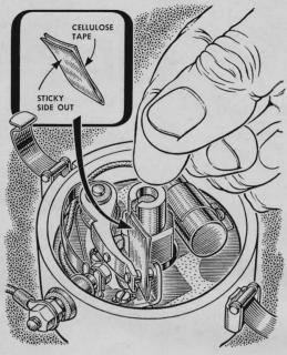
If you file breaker points, be sure all particles of metal or dirt are removed. One way of doing this: fold cellulose tape with the adhesive side out, press it between the points, bring them together. However, point replacement usually is best.
