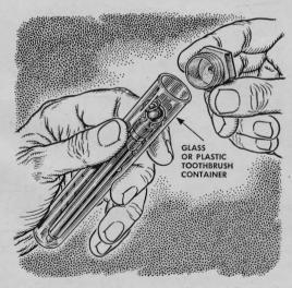
**Gauging tire pressure** regularly is a rule it pays every car owner to follow. For this, a reliable gauge is needed. One way of protecting the gauge is to store it in a toothbrush container. Dirt may damage a gauge carried loose in the car.
