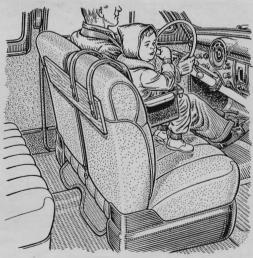
A baby seat hooked over the passenger seat of a two-door car may pitch the child forward in case of a sudden stop, if the driver is alone. To prevent this, screw the ends of the seat hooks to a board long enough to extend behind the driver's seat.
