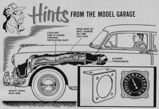
**Keeping track of air temperature** while you drive may offer a warning of icy conditions ahead, especially when it's near freezing. Here's the setup one driver installed,
