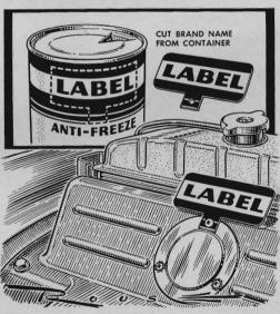
A durable antifreeze tag for attaching to the radiator can be made by cutting the brand name from an empty can. Paper tags ordinarily used to show what's being used and warn against draining have a habit of falling to pieces if they become wet.
