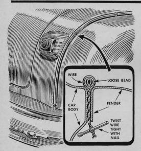
If the beading pulls away from the joint between body and fender, you can pull it back in place with a short piece of soft, noncorrosive light-gauge wire, perhaps Monel. Put a nail through the looped wire under the fender and turn to tighten.
