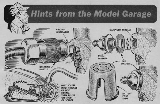
**Grease-fitting threads** may allow a serious loss of lubricant if damaged. One mechanic has found that this often occurs when new kingpins are installed. In such cases, he removes and heats the fittings, melts solder
