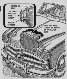
Flying stones can break head lamps and damage the radiator when you travel at high speed over the gravel roads that you find in some parts of the country. A piece of screening slipped down in front will protect the radiator core. Round pieces of screening taped over the lenses with wood spacers will take care of the glass.
