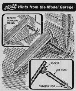
**Coupling springs** on the accelerators of Ford and International trucks sometimes break as shown in the upper inset. Because few dealers stock the springs, one garage operator gets the trucks back into service while waiting for delivery of factory replacements by installing a piece of air hose. The hose simply twists into place.
