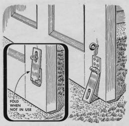
A hasp can be used to hold a garage door open. Screw it to the lower edge of the door so that the extended flap will dig into the ground as the door closes. Fold up the hasp and mount a screw eye in the slot to hold it up while not in use.
