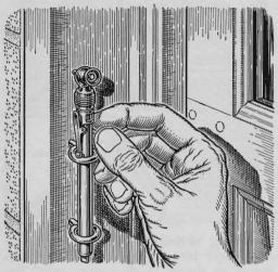
A tire-pressure gauge can only do its two important jobs (stretching tire mileage and tipping you to oncoming trouble) if you keep it where you can always find it for checking cold tire pressures. A pair of screw eyes in a garage wall make a handy rack.
