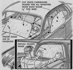
Cardboard shades fitted into the windows and windshield on the inside will help keep your car from heating up like a greenhouse when you must park in direct sunlight. Cut the shields about \%" too big. Spring them in place and they will stay put.
