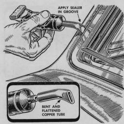
In applying sealer around a windshield, it is often difficult to press the fluid out of the tube without getting it all over the glass. A short piece of copper tubing placed over the end of the spout like this will help you do the job.
