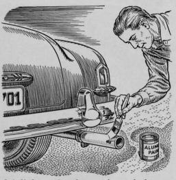
A tailpipe extension can be made from a piece of radiator hose. Force a piece of hose about 6" long over the end of the tailpipe and apply aluminum paint. Extend the hose beyond the bumper so that the chrome will be protected.
