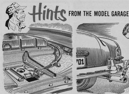
Copper tubing installed as a housing for flexible control cables running to hoodrelease mechanisms and heaters will eliminate lost motion and buckling. In the case of a hood release, the hold-down bracket can be placed over the tubing.
