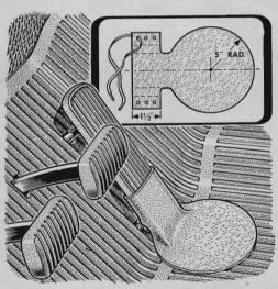
A rubber heel pad attached to the accelerator as shown above will stave off those unsightly holes in the floor covering. The pad can be cut from an old inner tube. Tie the end of it around the base of the accelerator pedal.
