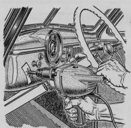
In drilling any part of the car metal to install accessories, first stick a piece of tape over the site of the proposed hole. Then centerpunch the hole and start drilling. With this precaution, the chance of damaging finish around hole is greatly lessened.
