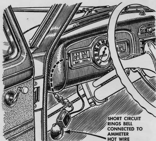
A short in the wiring of an old car is sometimes difficult to hunt down because it is intermittent and unpredictable. If that happens to you, try connecting a doorbell in series with the hot lead to the ammeter and systematically bouncing on the bumper and wiggling the wiring until the sound of the bell leads you to the short.
