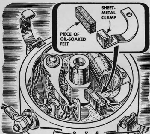
Ignition troubles are sometimes traced to rapid wear of the fiber rubbing block that actuates the ignition points in the distributor. This wear can be reduced by keeping the cam lubricated. A felt oiler held in a sheet-metal clamp is one way of doing this. Apply a drop or two of light oil to the felt.
