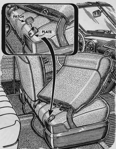
An annoying rattle may develop in the passenger seat of late-model Fords which have a small metal plate and limit bolt as shown here. The rattle usually can be eliminated by applying a ready-cut tire patch to the metal to act as a cushion.
