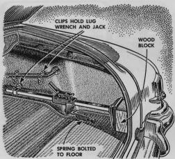
Rattle-free jack storage is easily provided. Attach two pipe straps to the trunk side with self-tapping screws, canting one in relation to the other so you'll have to press the wrench in place. Mount a spring to keep the jack butted against a wood block, with the shaft resting in a metal clip. Use the block as a wheel chock.
