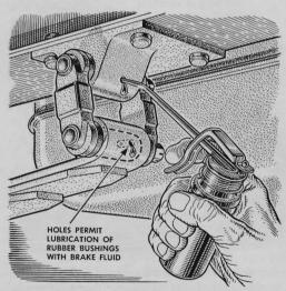
A persistent squeak in a rubber-bushed spring shackle usually can be eliminated by drilling a hole into the bushing and forcing in brake fluid with a pump oiler.
