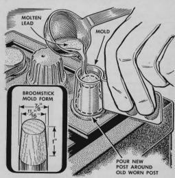
If a battery post is so worn the cable won't hold, cast a new post around the old one. Make a form by shaping aluminum around a broom handle tapered as shown.
