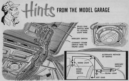
A lamp that lights automatically when you lift the trunk lid can be installed with parts that cost around a dollar. A mercury switch will take care of turning the light on and off. A flush-mounted clearance lamp with a clear lens is a good choice for the light. It usually can be set into a recess in the lid or body bracing by placing a metal
