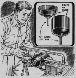
Two handy funnels for shop use can be made by sawing in two a throwaway type of oil filter. Remove the inside element. Thread two short pieces of %" pipe, screw them into the already threaded holes in each half, and the funnels are complete.
