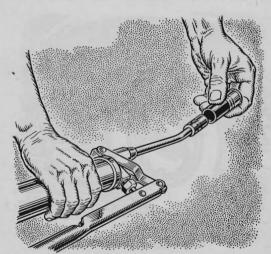
A used shotgun shell slipped over the nozzle of a grease gun will protect the coupling and keep out dirt. Dust and dirt that collect in the lubricant are sometimes driven into the grease fitting. A 12-gauge shell fits the nozzle snugly.
