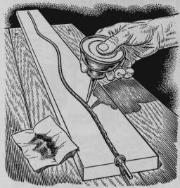
**Graphite** is the ideal lubricant for a speedometer cable, but getting it into the cable sheathing may be a problem. Here's one way of doing it: remove the inner cable, lay it on a board, apply the thinnest possible line of light oil on it, spray powdered graphite on the oil until the oil is blotted up and replace the inner cable.
