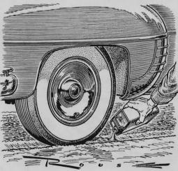
If sand is carried in a couple of one-gallon, screw-top cans, you can simply pour it under the tires when you get stuck on ice or snow. No need for a shovel to spread it. The cans are better than a box, for the sand can't scatter through the trunk.
