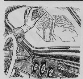
Windshield fog and steam can be wiped away quickly with a cellulose sponge. It will remove dirt and grease streaks and absorb considerable moisture before becoming saturated. A small inexpensive sponge will do the trick.
