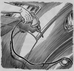
If water drips from the rain troughs and seeps into the trunk, you can divert most of it by simply closing the trough ends and drilling small holes an inch or so toward the front of the car. Close the troughs with solder or by squeezing them shut.
