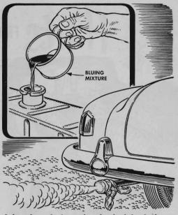
A head gasket can be checked for leakage by adding two spoonfuls of washing bluing to a cup of permanent antifreeze, pouring it into the radiator, tying a cloth over the tailpipe and running the engine. If there's a leak the bluing will color the cloth. The antifreeze will help you in locating the leaky trouble spot.
